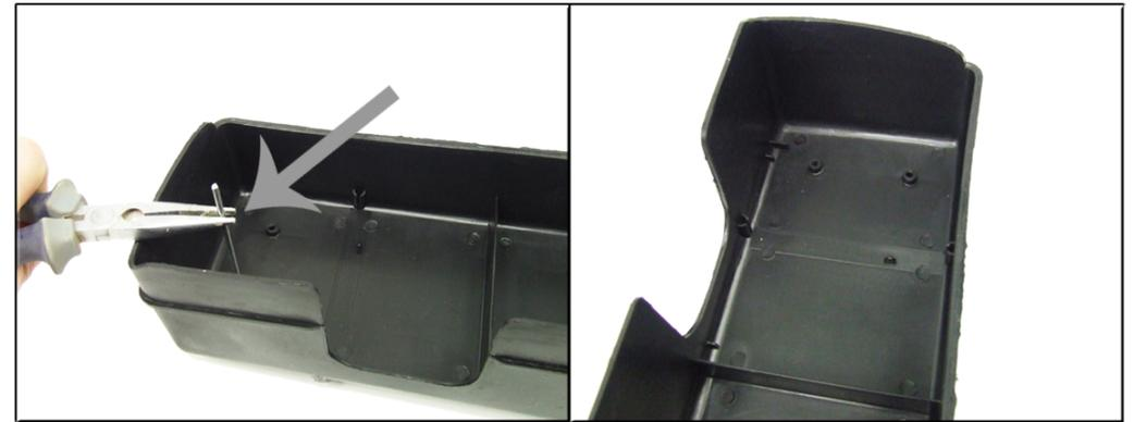
Using a pair of pliers remove the metal bait spike.
