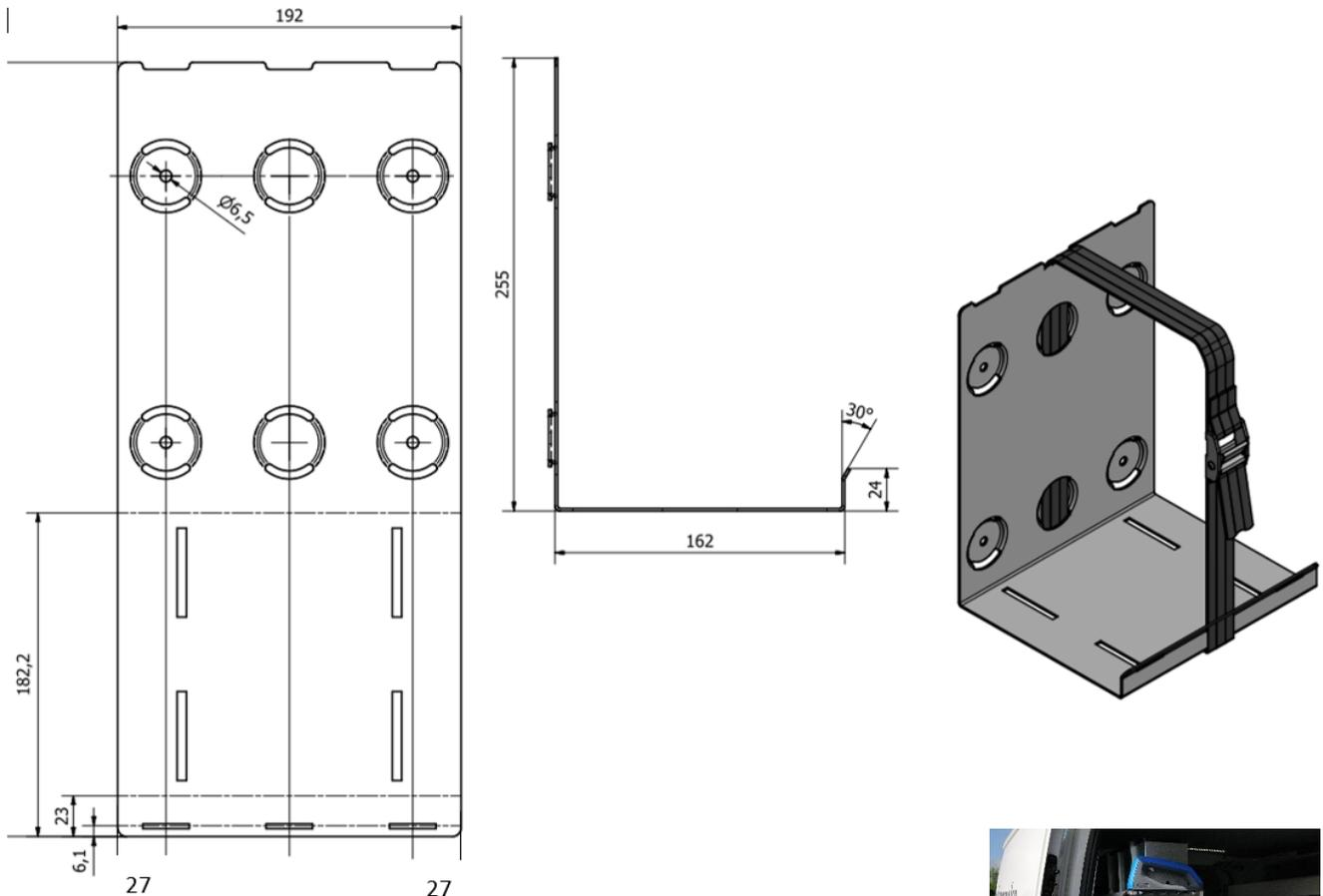
The bracket is supplied without screws and other accessories as the mounting should be adjusted to the individual mounting surface and conditions. Please note that mounting in a car should be done with special consideration to the construction of the car – contact your mechanic or an authorized garage.
